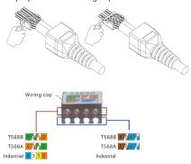
5. Place the wiring cap onto plug, use plier to clamp wiring cap until it completely snap-in to effect the connection.
